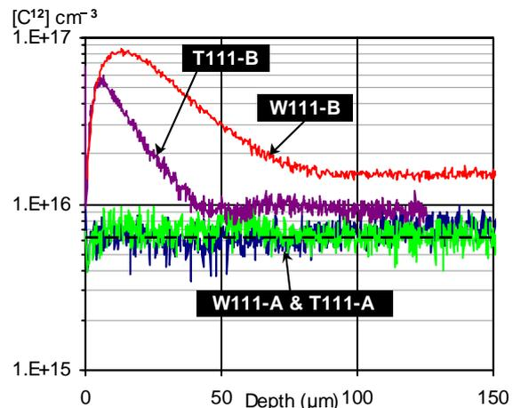
Fig. 4: Carbon concentration on <111> samples with and without TCA.
