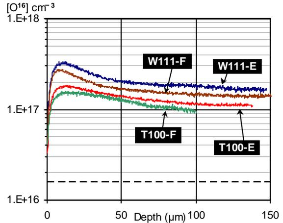
Fig. 3: Differences in oxygen content between <100> and <111> samples and between SiC and quartz tubes.
