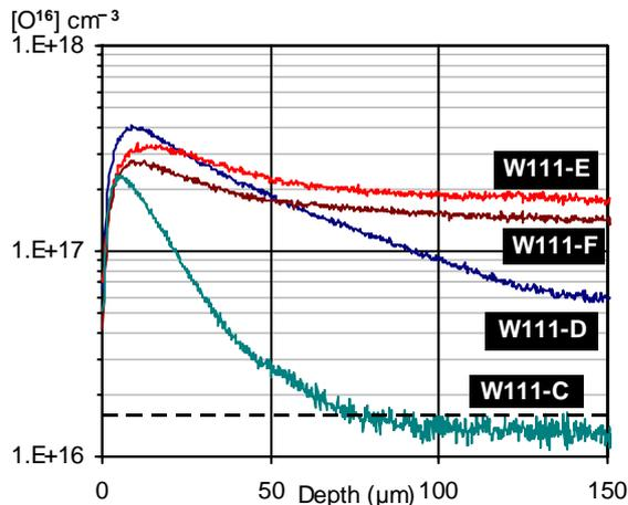
Fig. 2: Oxygen concentrations obtained with different processing times.
