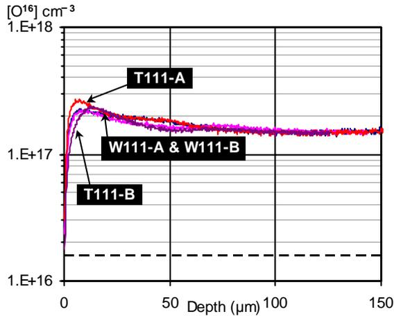
Fig. 1: SIMS Oxygen content on some <111> samples.
