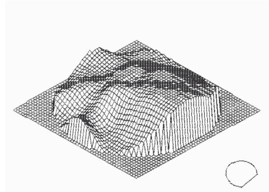
Fig. 7: Four point resistivity measurement after thermal processing.
