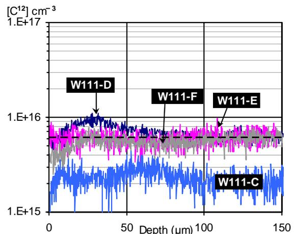
Fig. 5: Carbon concentration on <111> samples processed in quartz and SiC tubes.
