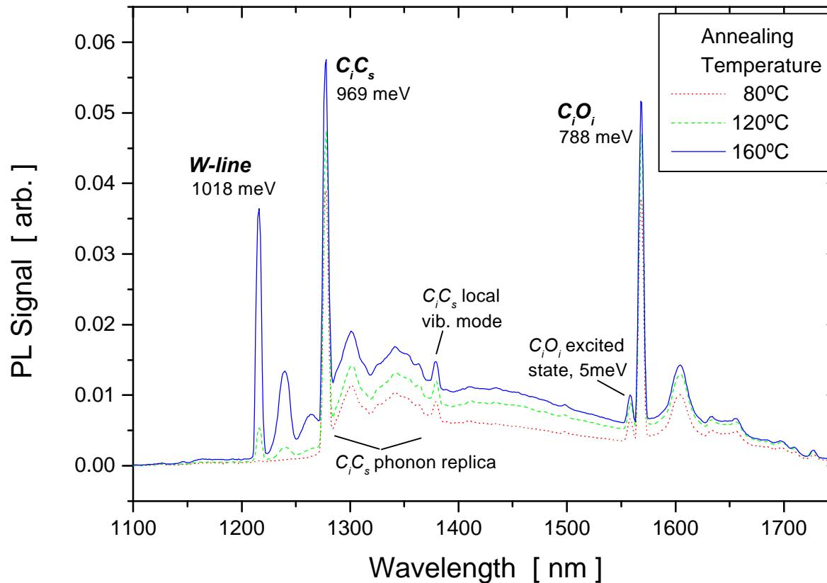
55 MeV proton irradiated standard silicon ( $5 \times 10^{13}$  p/cm<sup>2</sup>)
