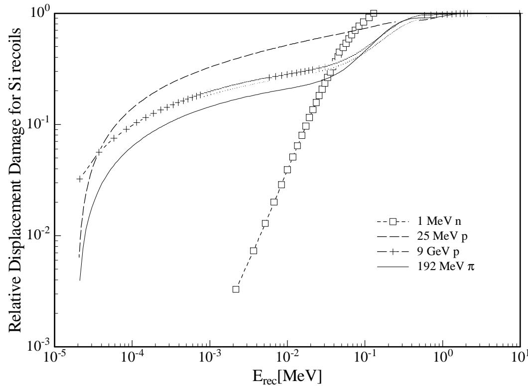
Relative damage produced by Si recoils with energies < 5 keV
