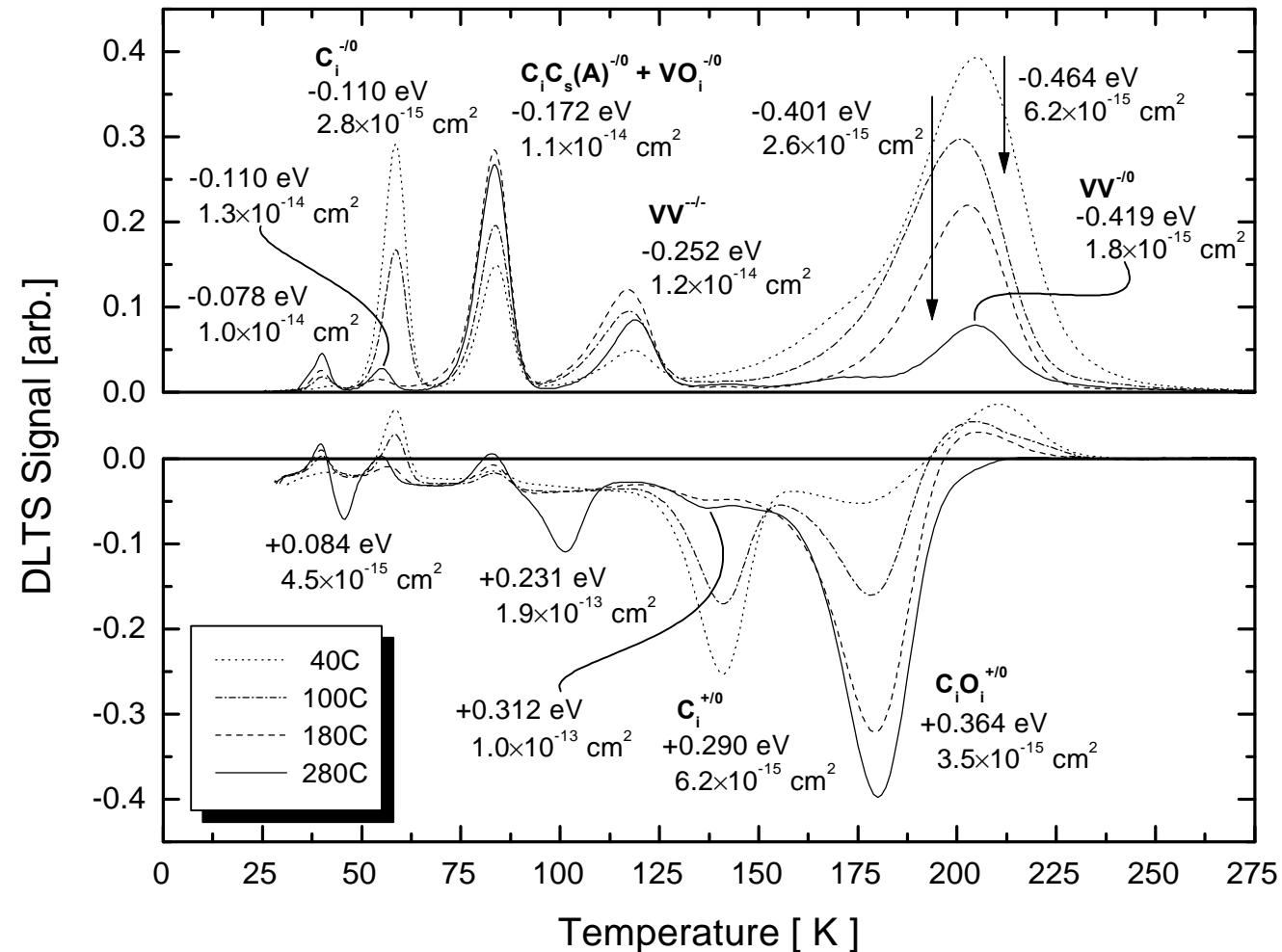
**Measurement of defect parameters:**
