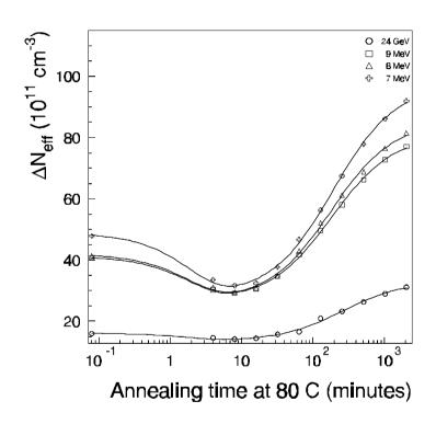
• Fluence:  $3.0 \times 10^{13} \text{ p/cm}^2 \text{ for } 7,8,9,10 \text{ MeV protons}$  $4.9 \times 10^{13} \text{ p/cm}^2 \text{ for } 24 \text{ GeV/c protons}$
